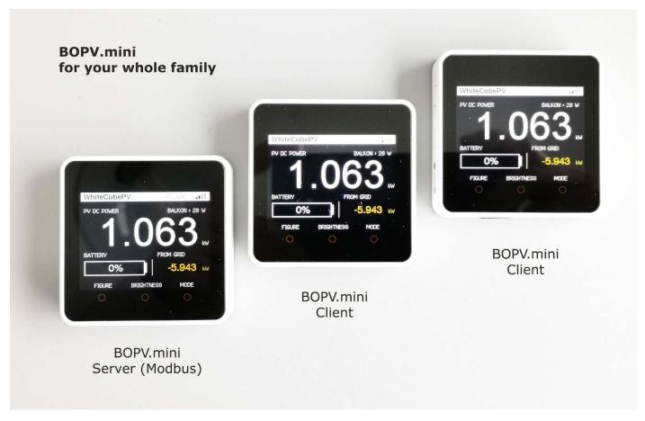
Set up the main unit normally as described in the instructions above. Add the option "IsServer=1" in the config .txt. This activates the internal web server. After that, more BOPV.mini can access it.
