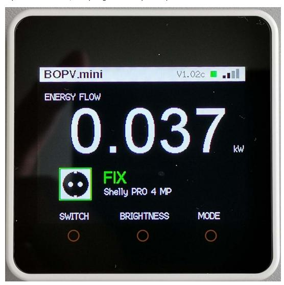
The setup is as simple as with family mode: "FromServer=IP" is the IP address of your meter (myStrom Switch or Shelly). "ServerType=x" refers to the device that provides the data.
