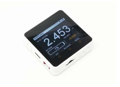
The dimensions of the device are  $54 \times 54 \times 16$  mm. This means that it has the size of standard switch ranges and can be integrated in an optically excellent manner.
