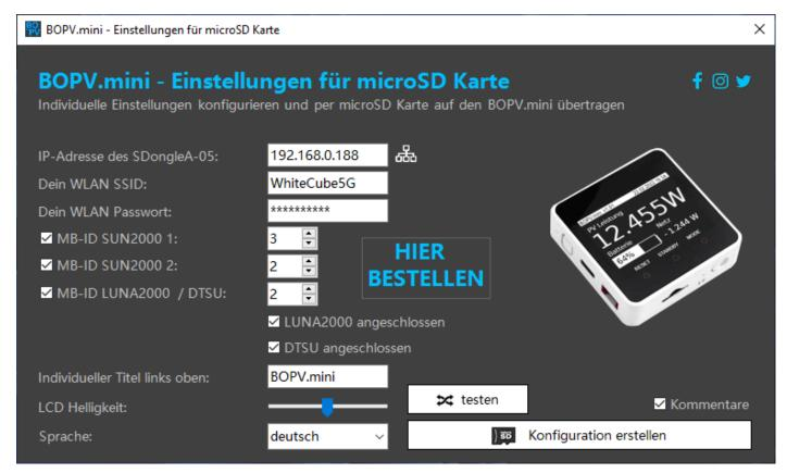
The configuration file is created automatically with "Create configuration". Copy this to the micro SD card and then insert it into the BOPV.mini before switching it on.
