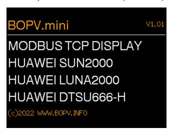
Next, it is checked whether a micro SD card is inserted and whether the config.txt file is on it. If there is a problem here, 2 beeps will sound and a message will appear on the screen. Now the BOPV mini tries to connect to your WLAN. If the parameters on the SD card are correct, the connection parameters are displayed. Otherwise, three beeps will sound and a message will appear on the screen.
